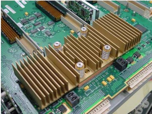
Fig. 14 Cross Bar Chip Heatsink
