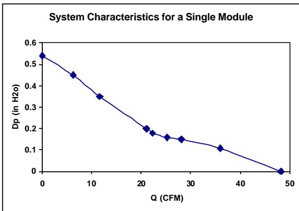
Figure 5. Pumping-type overall characteristics for the forward flow through a passage
