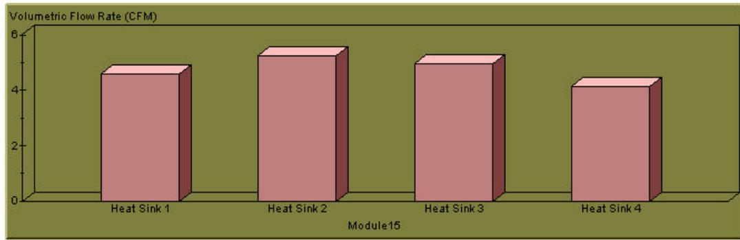
Figure 11. Flow rates through the heat sinks in 15<sup>th</sup> passage (out of 20) for an isolated cabinet.
