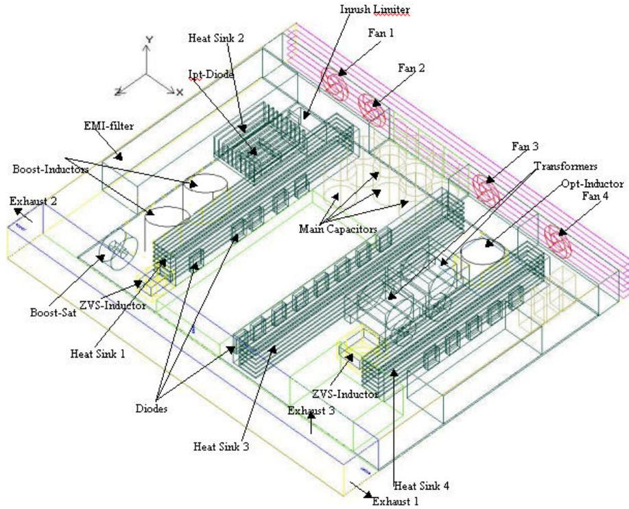
Figure 1. Schematic diagram showing the arrangements of components on a single board
