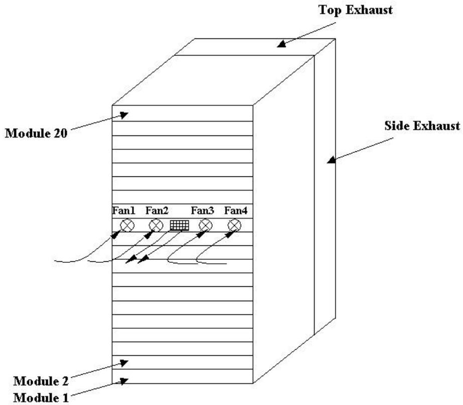
Figure 2. Schematic diagram showing the arrangements of the boards in the power system cabinet.
