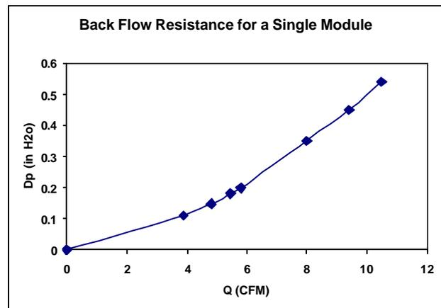
Figure 6. Resistive-type overall characteristics for the reverse flow.
