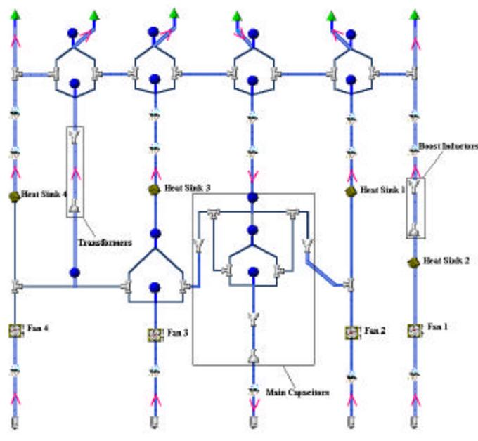
Figure 4. Flow network model for a single passage
