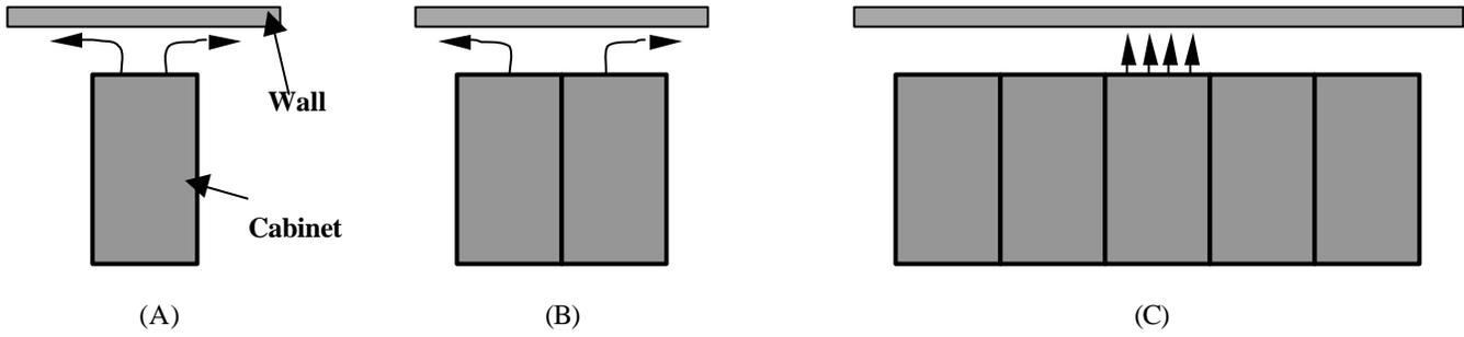
Figure 3. Three different placements of the power system cabinets analyzed in the present study
