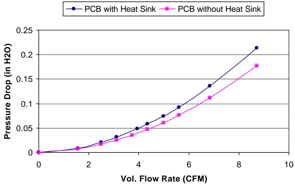
Figure 3 – Impedance characteristics of the card passages determined using CFD
