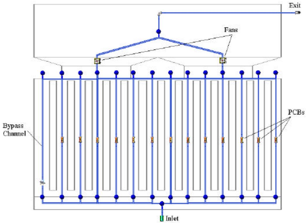
Figure 4 – Flow network representation of the flow through the cabinet
