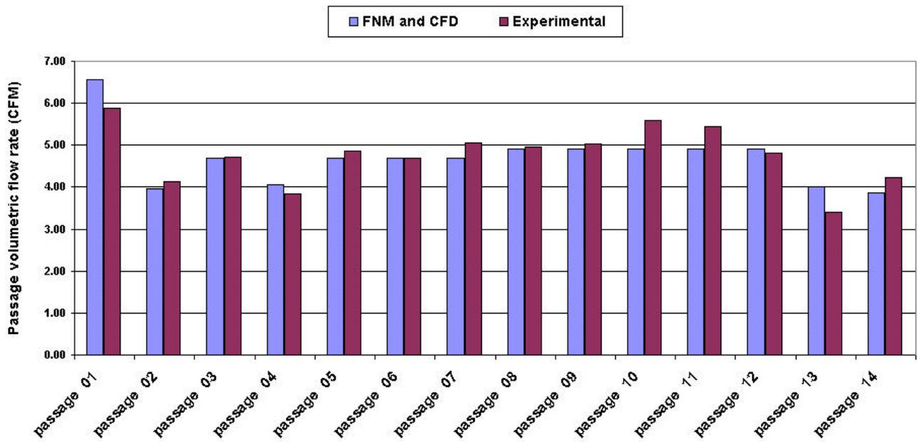
Figure 5 – Variation of the volumetric flow rates through the card passages and its comparison with experimental measurements
