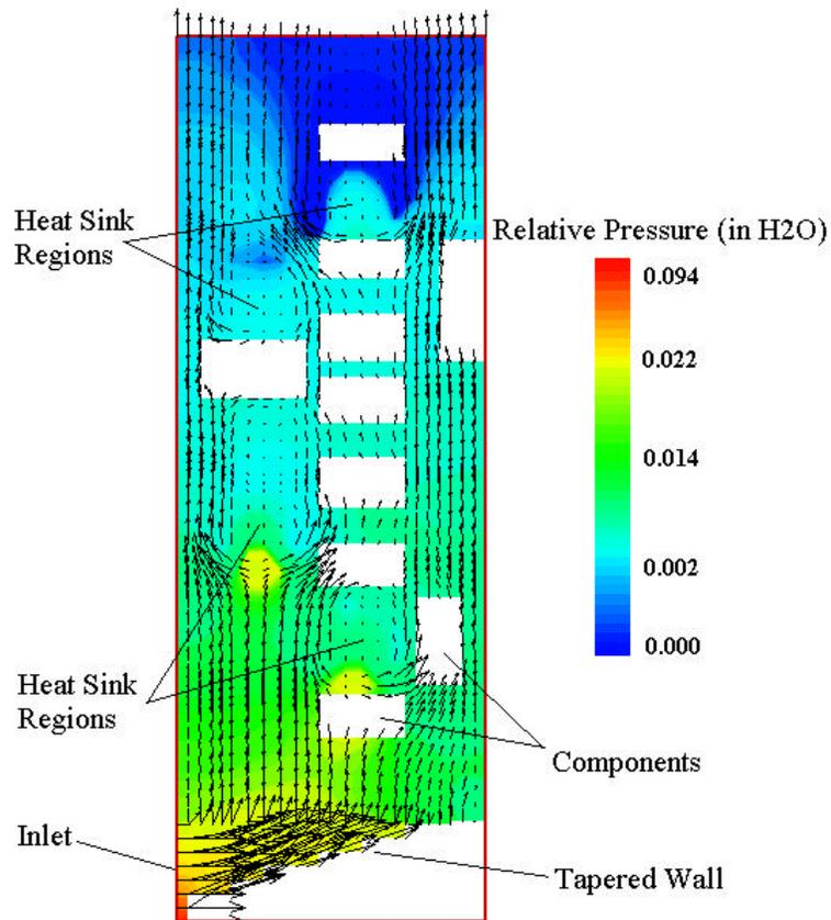
Figure 6 – Velocity vectors and the pressure contours in a plane through a card passage.
