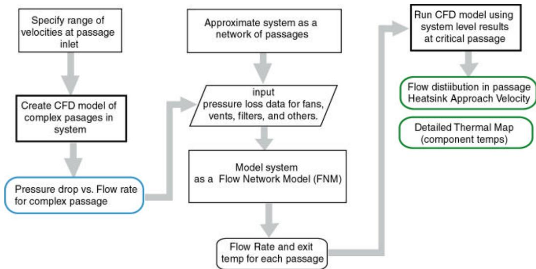
Figure 2 – Flow chart of the analysis technique used the
