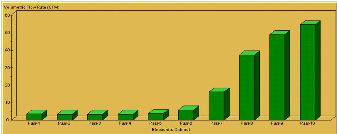
Figure 3. Volumetric flow rate through card passages for Design I
