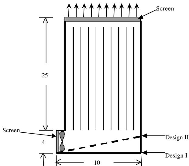
Figure 1 – Layout of the electronic cabinet
