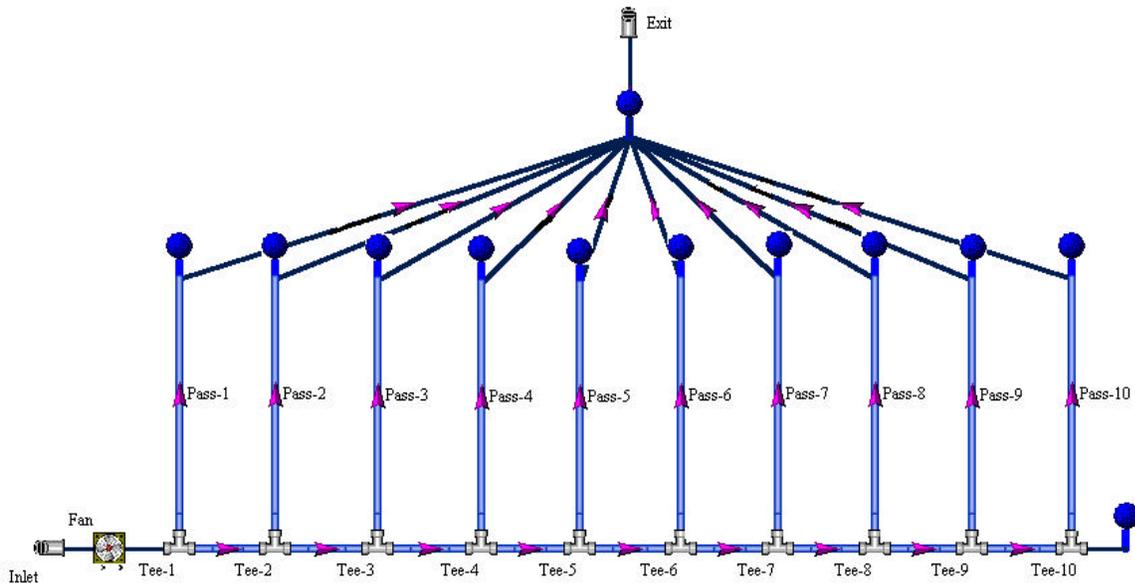
Figure 2 – Flow network representation of the electronic cabinet
