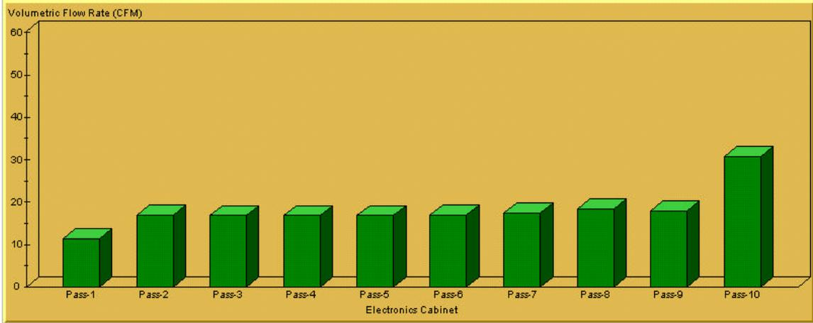
Figure 4. Volumetric flow rate through card passages for Design II
