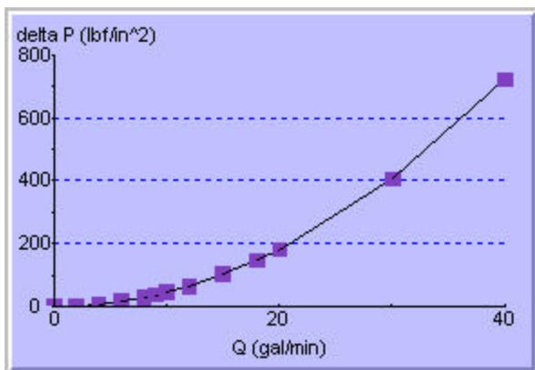
Figure 6. Pressure-Flow Piecewise Linear Correlation for Resistance Element
