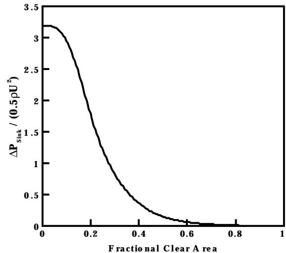
Figure 5 – Variation of the pressure drop through the heat sink as a function of the fractional clearance area around the heat sink.
