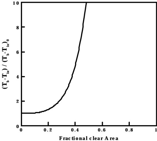
Figure 6 – Variation of the base temperature of the heat sink as a function of the fractional clearance area around the heat sink.
