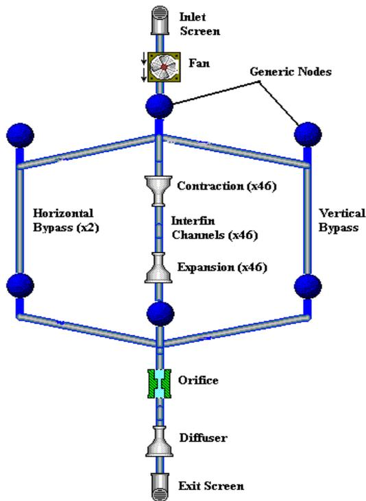
Figure 3 – Network representation of the test cell used characterizing the heat sink performance
