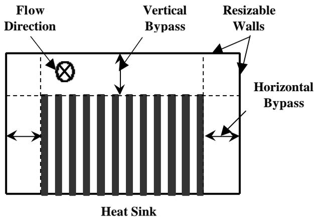
Figure 2- Cross-sectional view of the heat sink with bypass
