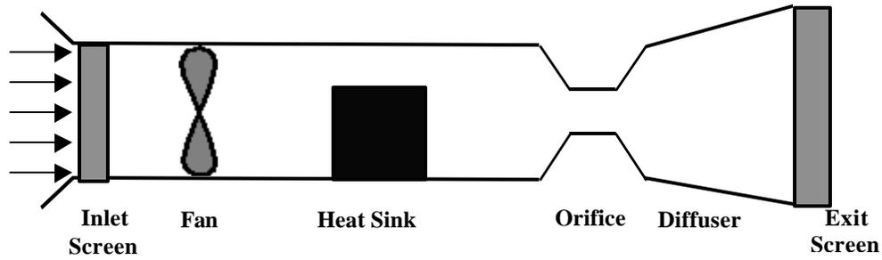
Figure 1 – The wind tunnel test cell for characterizing heat sink performance
