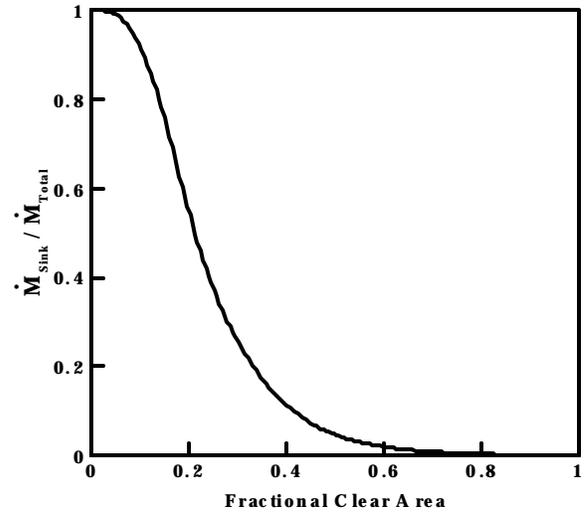
Figure 4 – Variation of the fraction of the total flow through the heat sink as a function of the fractional clearance area around the heat sink.
