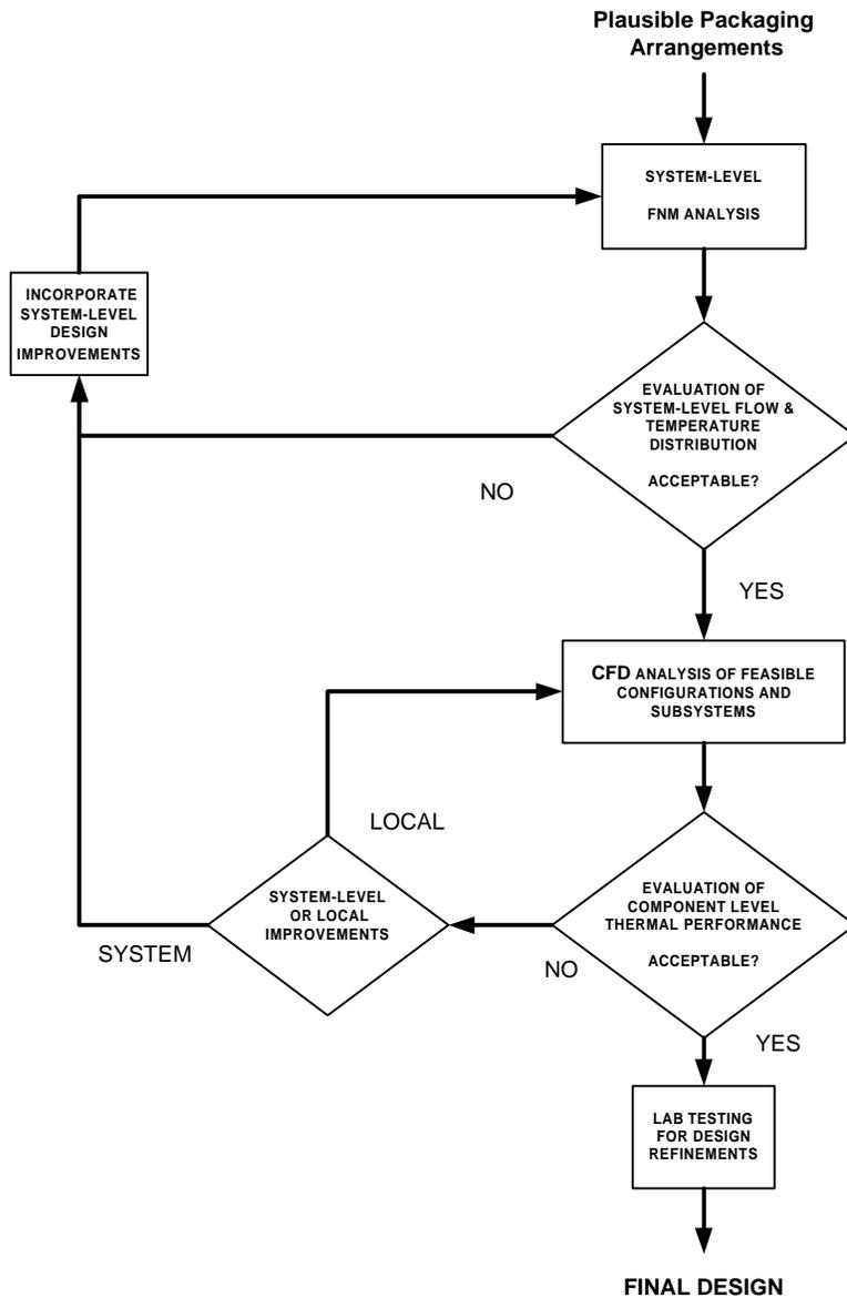
Figure 5 – The enhanced design cycle incorporating Flow Network Modeling (FNM) for system-level design
