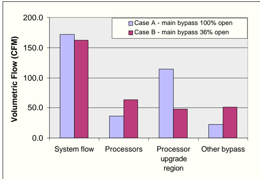
Figure 3 – Correction of flow imbalance between processors and the main bypass region
