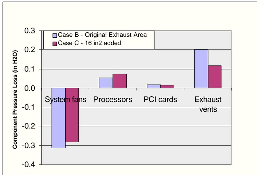
Figure 4 – Effect of the reduction of the flow impedance at system exhaust
