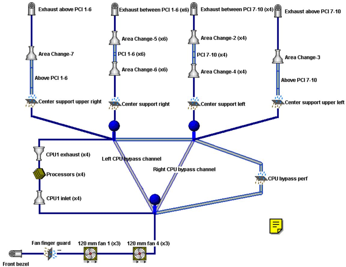
Figure 2 – Flow network representation of the air-cooled server
