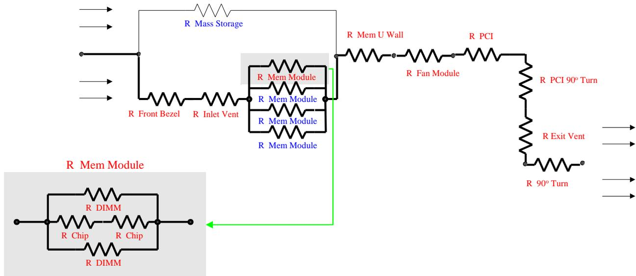
Figure 6: Detailed PCI/Memory Section Flow Network
