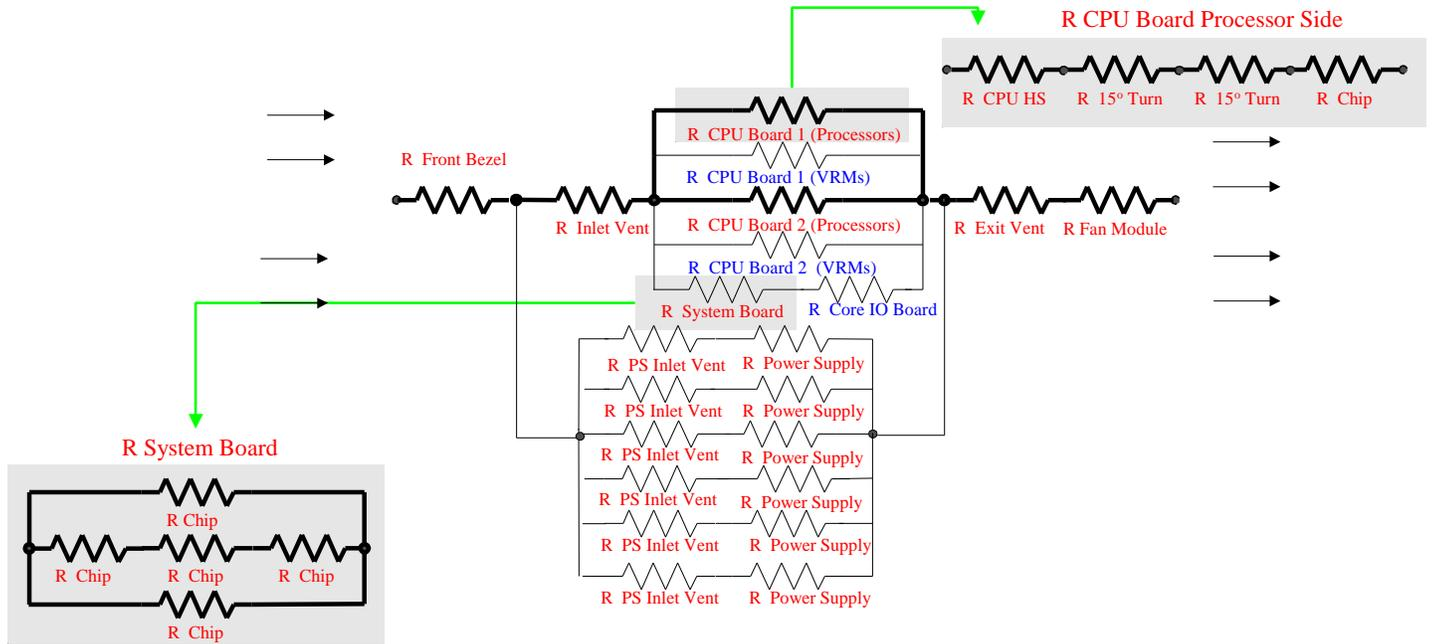
Figure 5: Detailed CPU/Power Section Flow Network
