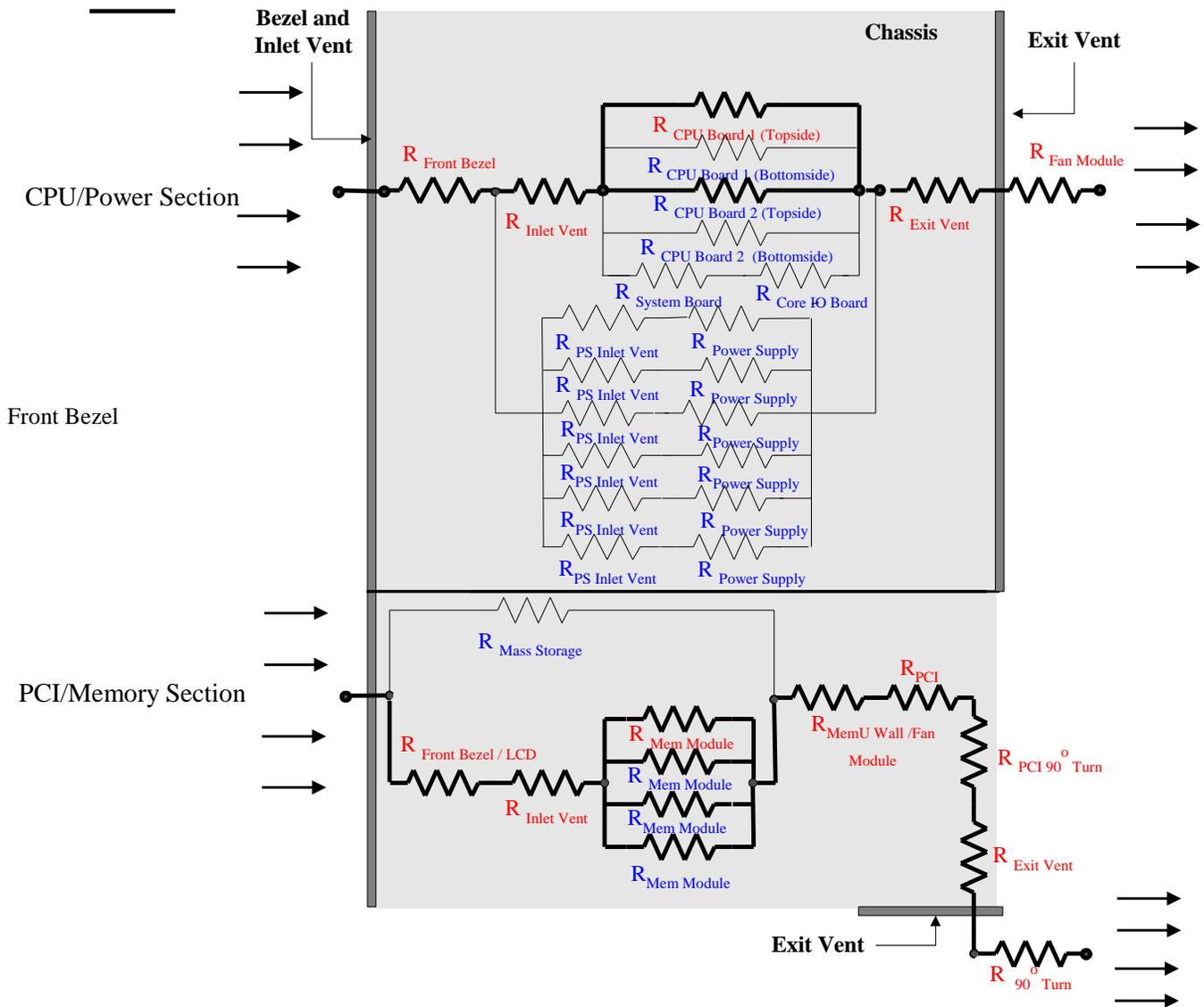
Figure 4: Flow Network Representation of a Future Computer System
