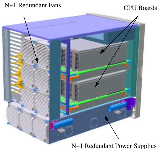
Figure 2: Computer System CPU/Power Section
