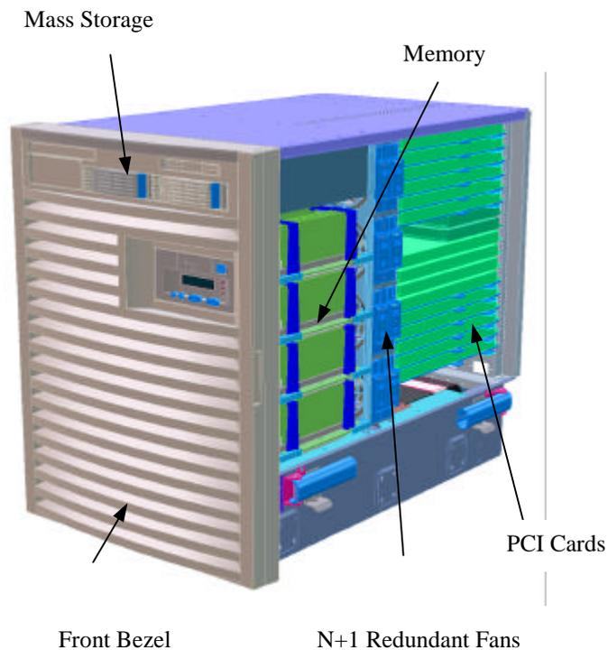
Figure 3: Computer System PCI/Memory Section
