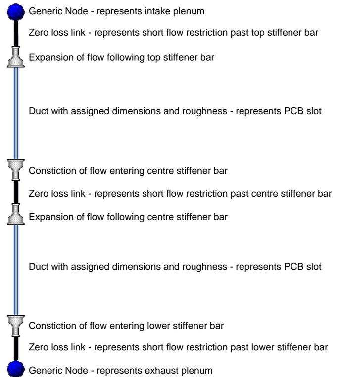
Figure 4. Enhanced Card Slot Model.
