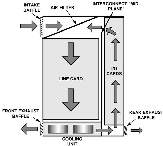
Figure 2. Partial Recirculation Cooling System
