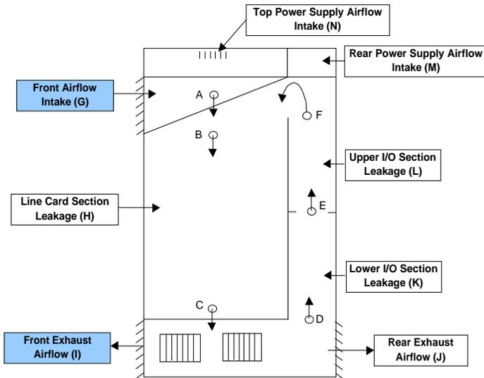
**Figure 7. Overview of system showing various volumetric flows**
