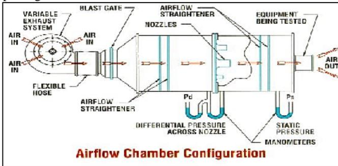
Figure 1. Airflow Test Chamber (Airflow Developments, Inc.)
