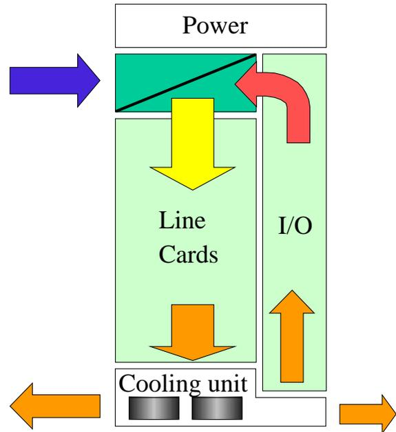
**Figure 5. Direction of Flow in 50 Gig System.**
