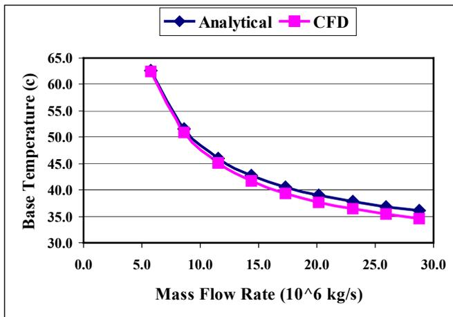
Figure 9. Average base temperature for HSAR2
