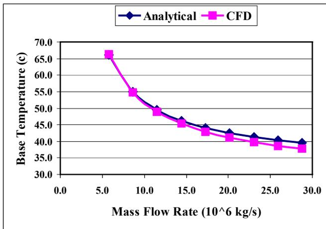
Figure 8. Average base temperature for HSAR1
