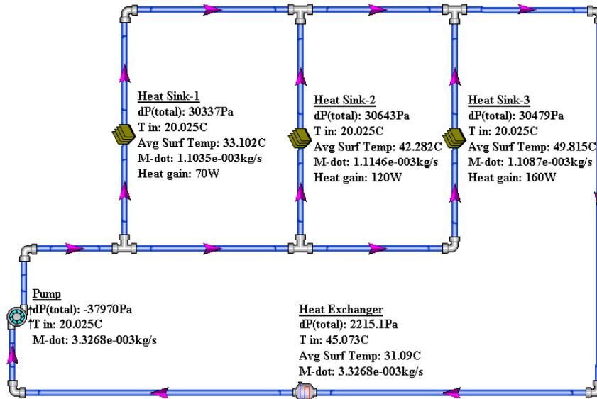
Figure 13. FNM model of the original liquid cooled system
