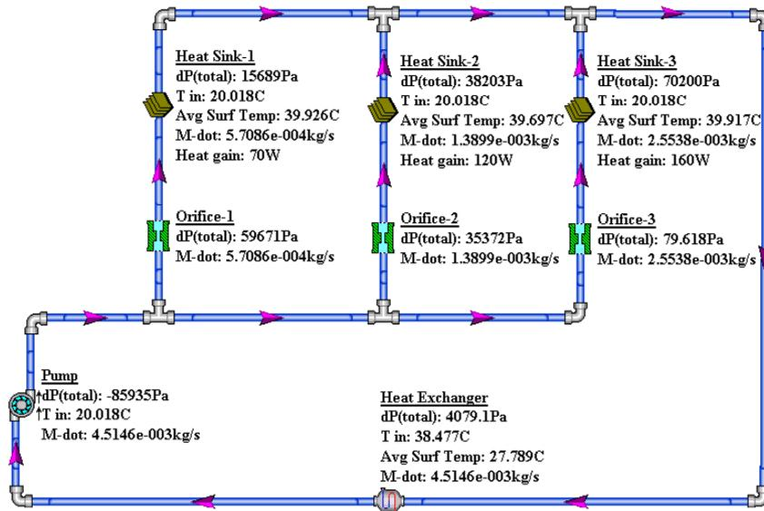
Figure 14. FNM model of the modified liquid cooled system
