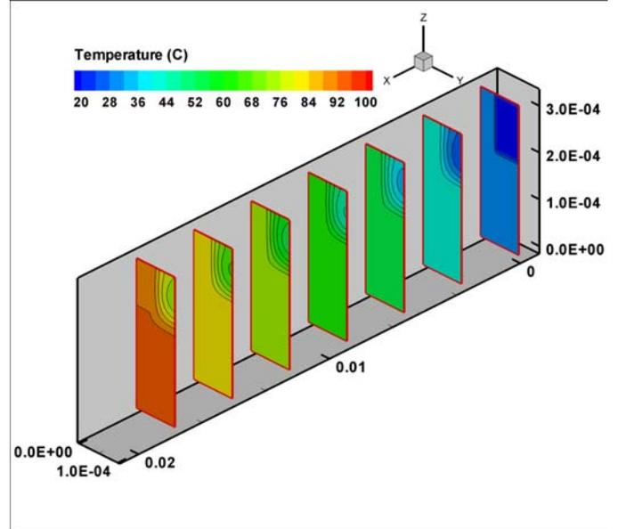
Figure 6. Temperature distribution inside HSAR1 at yz planes.
