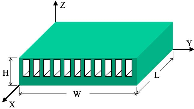
Figure 1. The schematic and overall dimensions of the microchannel heat sink (The drawing is not to scale)
