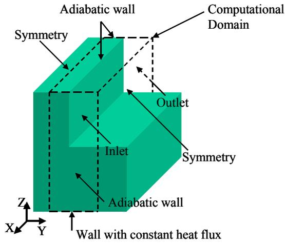
Figure 3. The computational domain and boundary conditions
