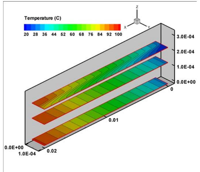
Figure 7. Temperature distribution inside HSAR1 at xy planes
