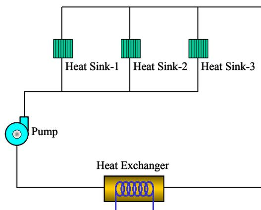
Figure 12. A liquid cooled system
