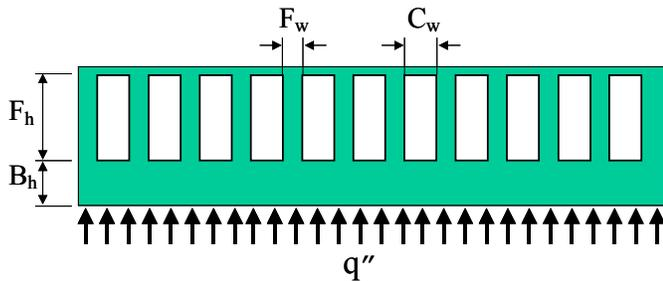
Figure 2. Dimensions of the microchannel heat sink (The drawing is not to scale)
