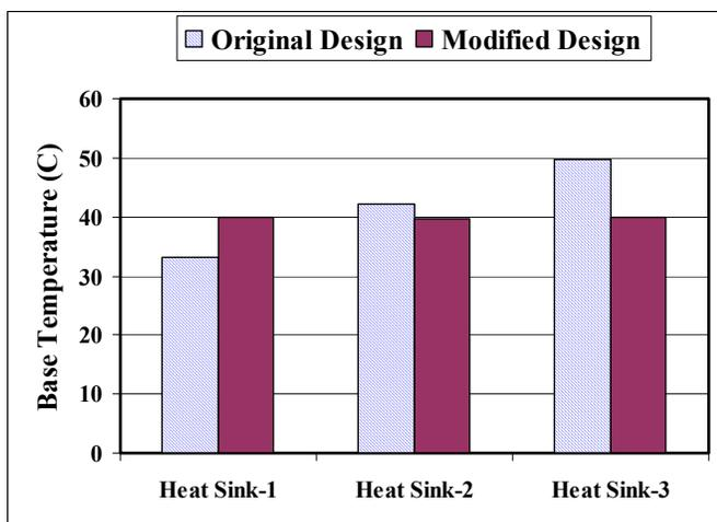
Figure 16. Heat sinks base temperature
