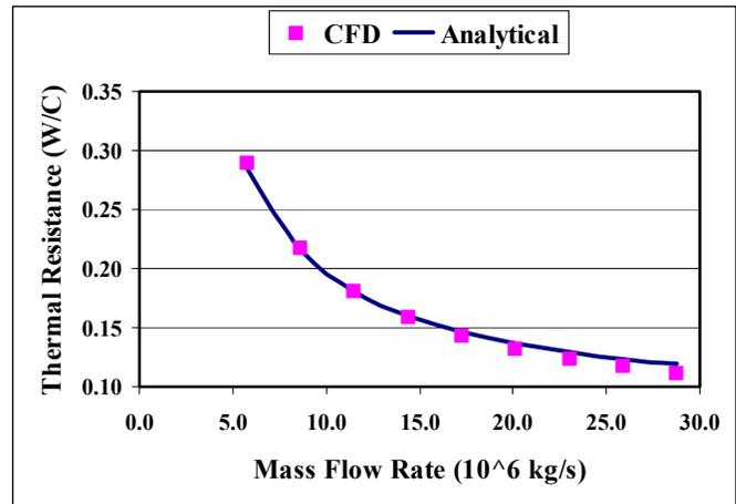
Figure 10. Thermal resistance for HSAR1
